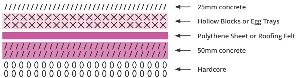
Polythene sheeting helps prevent damp rising through the floor and hollow bricks or egg trays provide insulation.
